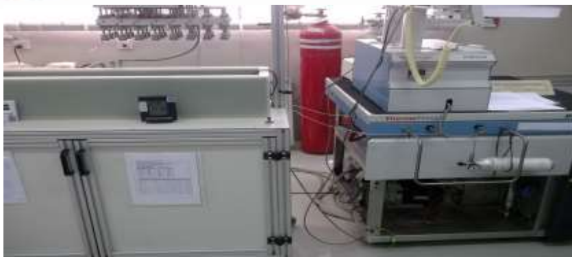
Mass Spectrometer (Determination of Stable Isotopes , O18 and Deuterium)
