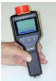
Handheld portable gamma-ray detector HM-5
