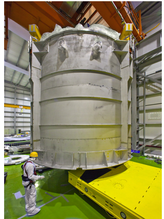
A detector tank, prior to installation at Daya Bay. (Photo by Roy Kaltschmidt/Berkeley Lab)
