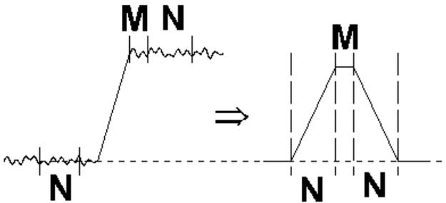
Figure 2. Typical trapezoidal weighting function (right) arising from detector preamplifier output signal (left).
