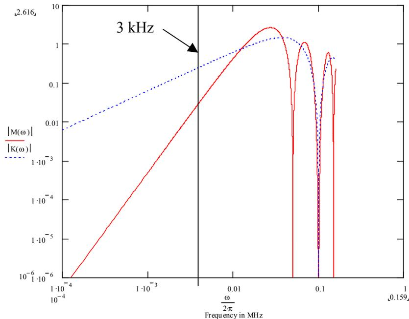
**Figure 5. Theoretical output of typical (dashed line) and LFR (solid line) weighting functions using 10  $\mu$ sec rise times.**
